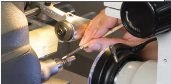
Precision winding techniques performed with the aid of a microscope.
