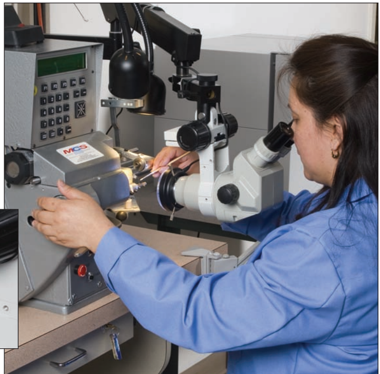
Precision winding techniques performed with the aid of a microscope.
